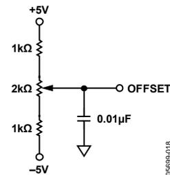
Figure 20. Circuit to Control  $V_{OFFSET}$  (±2.5 V)
