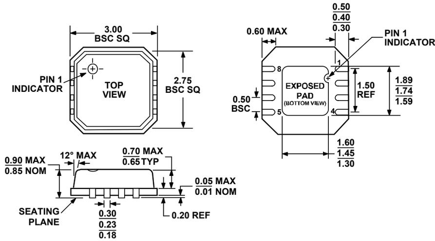
Figure 22. 8-Lead Lead Frame Chip Scale Package [LFCSP\_VD]
