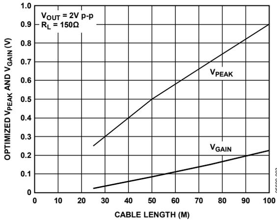
Figure 4.  $V_{\text{PEAK}}$  and  $V_{\text{GAIN}}$  Settings vs. Cable Length
