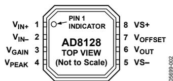
Figure 3. Pin Configuration
