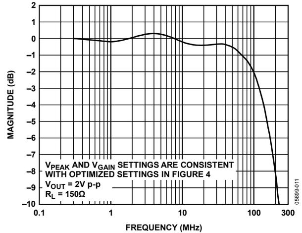
Figure 8. Equalized Frequency Response for 100 M Cable
